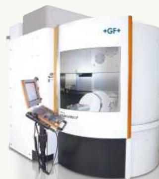
With its linear direct drive, the high-speed machining center Mikron HSM 600U LP is designed for maximum precision and surface quality.
