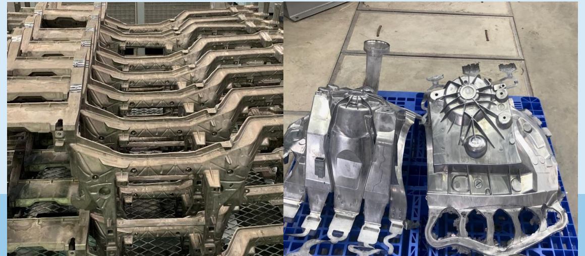
First test run successfully completed in September 2021 (Left: Cross Car Beam | Right: Shock tower)
