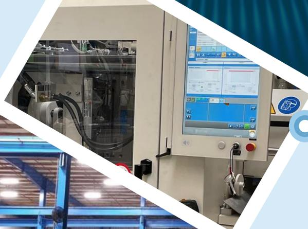
Focus on **energy efficient capex** – electric injection molding machine at GF Piping Systems in Schaffhausen (Switzerland)
